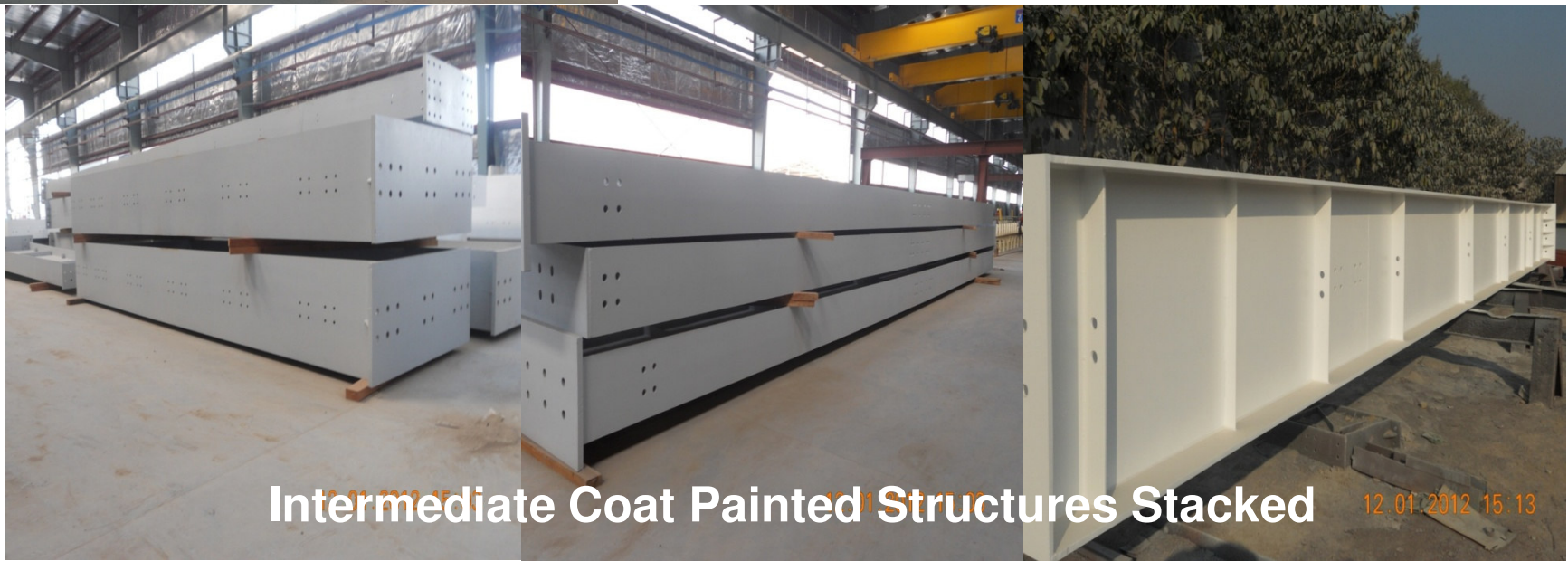
Crane Beam with web depth of 2.2 Metres
