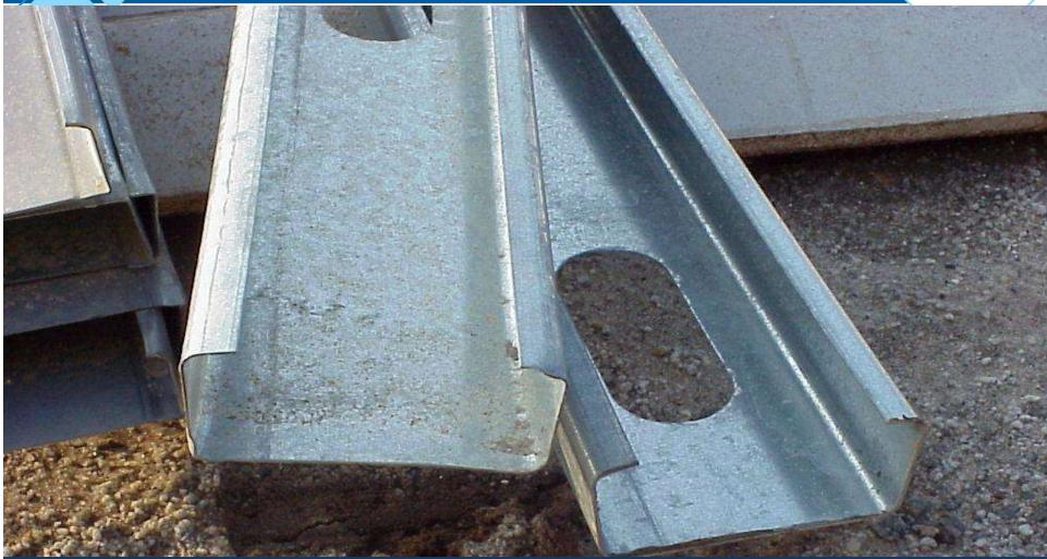
Cold rolled studs and joists are formed in "C" shapes, which provides lateral strength for studs and vertical strength for joists and rafters.
