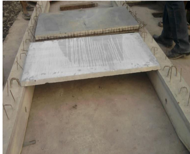
Normal stone broke instantaneously
