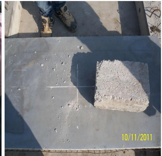
Surface after impact (completely intact)
